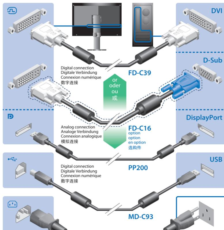
\*The USB cable is required for calibration. Be sure to connect the monitor and PC with the USB cable.
